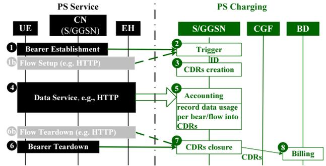
Figure 2: Charging procedures for a data service flow.
