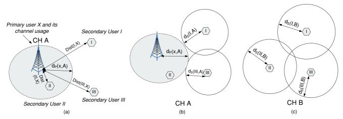
Fig. 1 Spectrum availability changing with the presence of primary users. (a) Topology (b) availability of channel/color A; (c) availability of channel/color B
