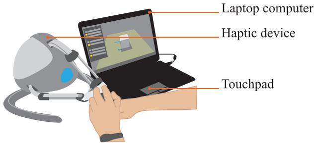
**FIGURE 2** Elements of the visuohaptic simulation
