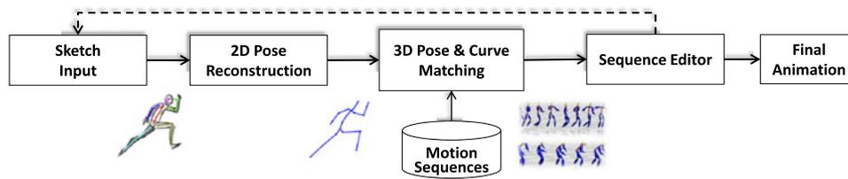
**Fig. 2** The overall schema of our framework. A user-defined 2D sketch is converted into a 2D annotated pose that is matched to a 3D pose from a large database. A segment of the sequence containing the detected pose is then used in the sequence editor to compose the final animated scene
