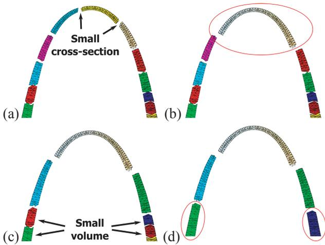
**Figure 4:** Pre-merging connects segments that would be difficult to assemble such as tiny cross-sections and small volumes: (a) shows the initial segments; (b–d) show segments merged while increasing the smallest segment volume and cross-sectional area.
