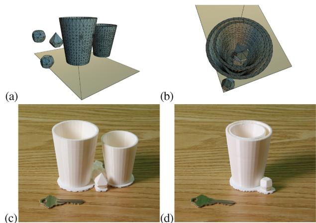
**Figure 13:** A sample packing of groups of objects: (a) shows the initial, random placement of objects, (b) packed configuration and (c,d) printed results. Note that the two crystals have been placed inside the smaller cup and the smaller cup inside the larger cup.
