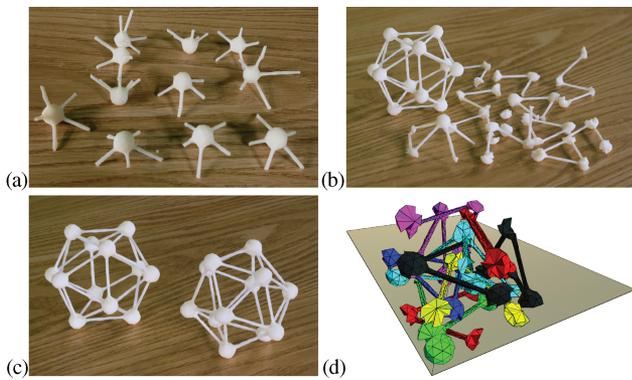
**Figure 11:** The model was first segmented without considering the cross-sectional area resulting in a model that was impossible to assemble (a). The model was segmented again with the gluing area considered, optimized, printed (b) and assembled (c); (d) shows the printing tray with the packing configuration (almost 40% savings of material).
