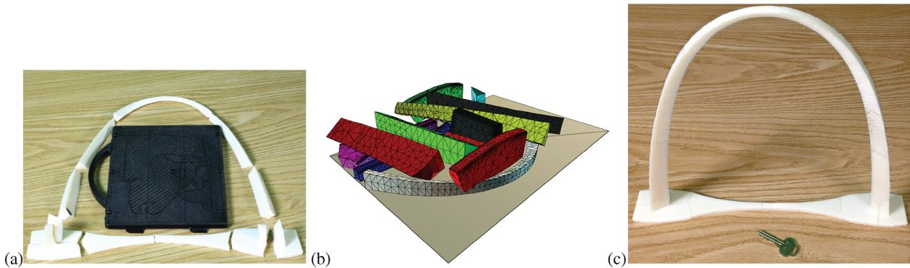
**Figure 9:** An object larger than the printing tray (shown in the figure) (a) was automatically segmented into pieces that fit the tray (b) and it was printed in a single print (b). It was then assembled in less than 5 min (c).
