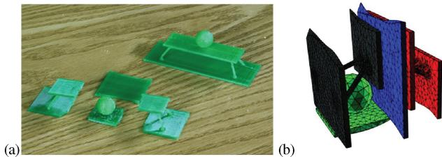
**Figure 12:** Example of printing on an FDM printer: Packed configuration (b) and the printed object (a).
