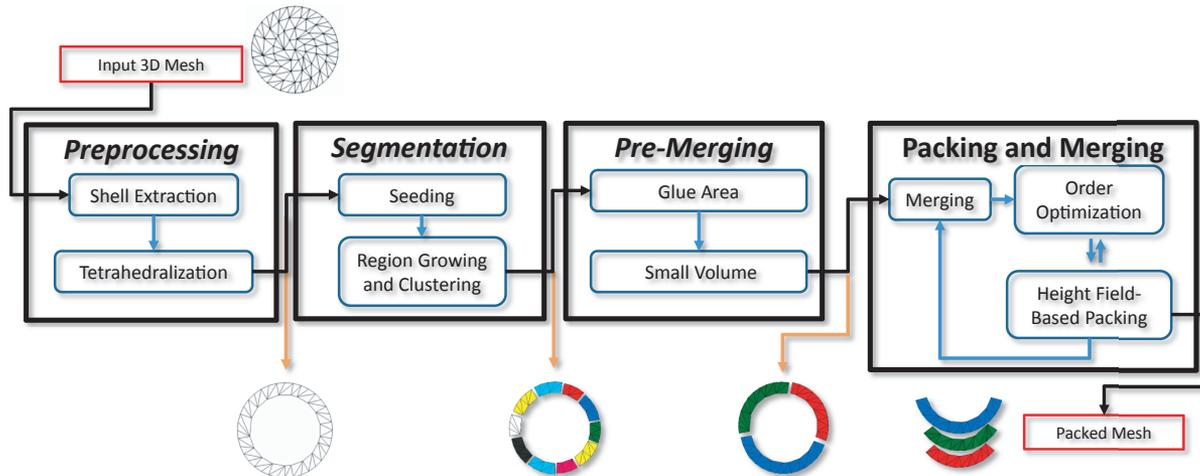
**Figure 2:** System overview. The input 3D mesh is pre-processed and converted into a volumetric shell. The shell is divided into a set of segments that are pre-merged, if they would cause problems during final assembly (small volume or small cross-sectional area). The updated segments are then tightly packed and merged together, resulting in a printing configuration that saves supporting material and speeds up the printing.
