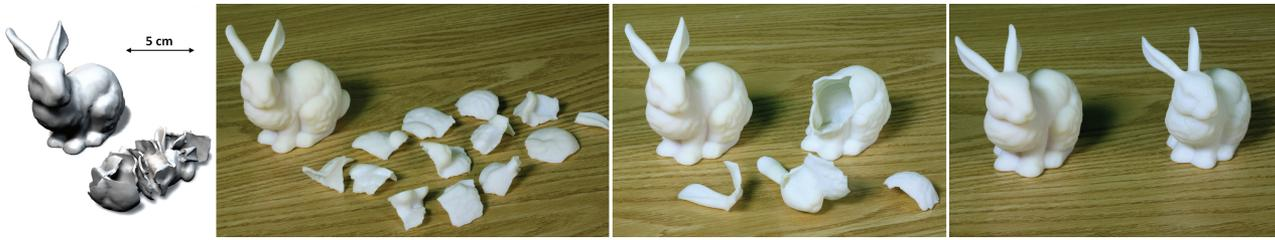
**Figure 1:** A 3D object was automatically divided into a set of similarly sized segments that can be easily assembled together and printed. The overall printing time was reduced from 13.5 h to 9.5 h (saving 30%) and the amount of support material was reduced from 351 g to 229 g (saving 34%). The optimization was completed in approximately 1 min and the final object assembly took about 15 min.
