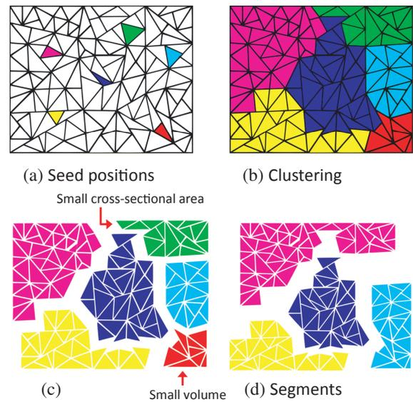
**Figure 3:** Segmentation first finds suitable seed positions (a) that are used to cluster the tetrahedra to near-to-equal segments (b). In the pre-merging step small segments are merged (c) resulting in a set of segments covering the input object (d).
