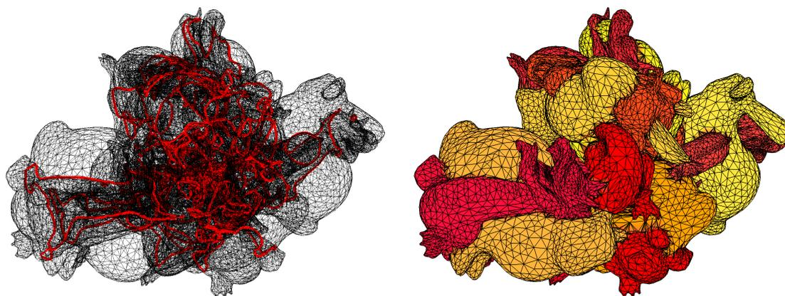
Figure 1: Six Stanford dragons and six Stanford bunnies (Levoy et al., 2005) intersect in 172 separate intersection boundaries (left). The final merged mesh (right) does not contain any intersections.
