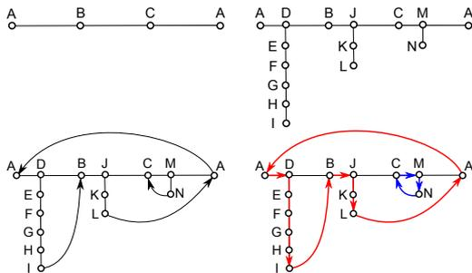
Figure 10: Left to right, top to bottom: list initiation; insertion of polylines; linking end points; polygon tracing.
