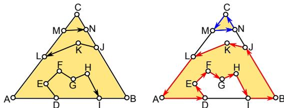
Figure 9: Polygon reconstruction. Intersecting polylines (left) and newly created polygons (right).
