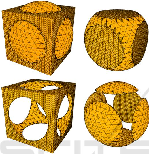
Figure 13: Boolean operation on cube  $A$  and sphere  $B$ . Left to right, top to bottom:  $A \cup B$ ,  $A \cap B$ ,  $A \setminus B$ , and  $B \setminus A$ .
