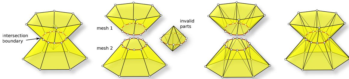
Figure 2: Left to right: intersection boundary detection, invalid parts elimination, polygon triangulation, and mesh stitching.
