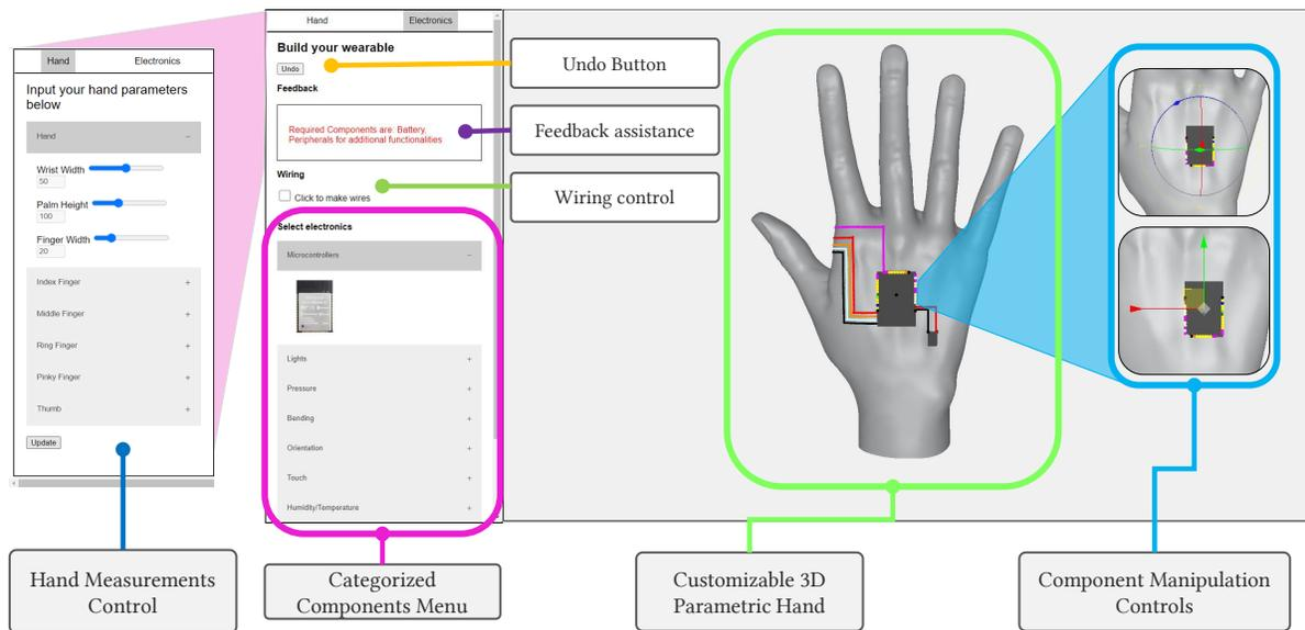
Fig. 2. FabHandWear Design Interface - Sections Description
