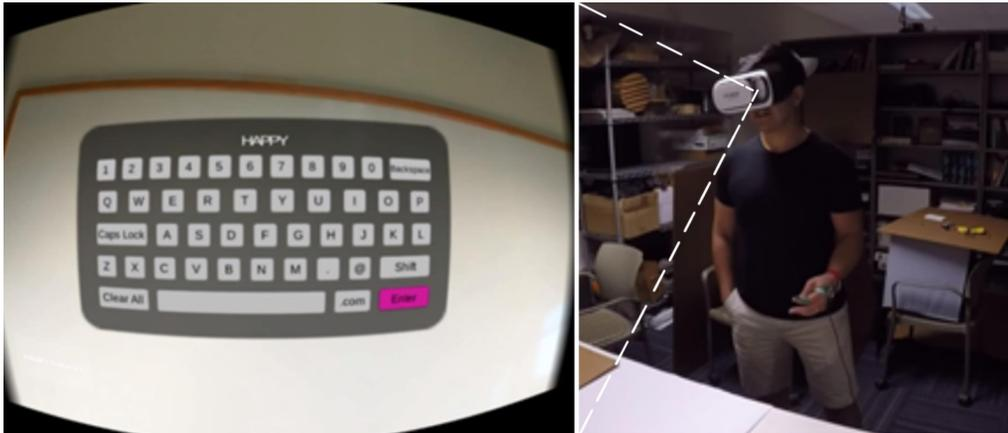
Fig. 3. A participant typing on a head mounted display using a hand wearable
