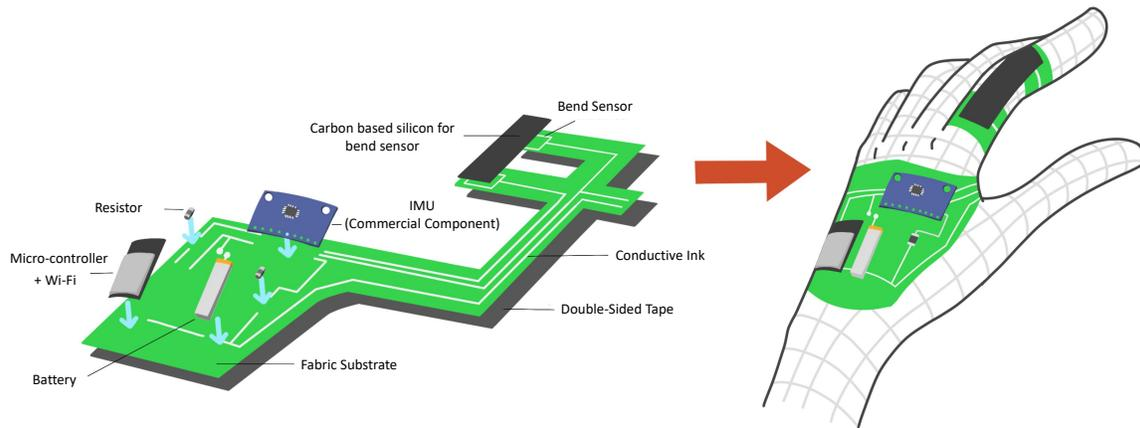
Fig. 6. FabHandWear System characteristics
