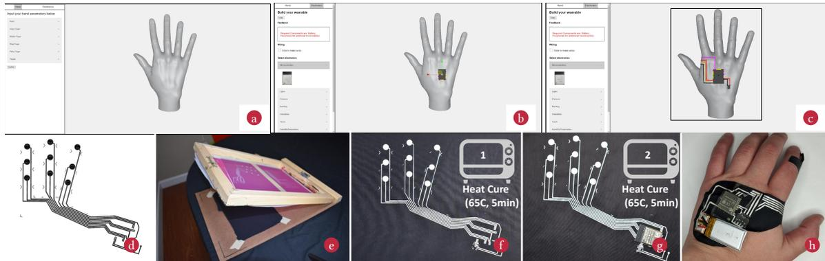
Fig. 5. Design and Fabrication Workflow: (a) Hand measurements parametrization, (b), Place desired components on the 3D handmodel, (c) Generate circuit wires (manually or autorouting), (d) generate and Print the template, (e) Screenprint circuits on nylon fabric using conductive silver ink, (f) heat cure the ink, (g) Assemble components on the circuit and heat cure the connections, (h) Hand wearing the prototype
