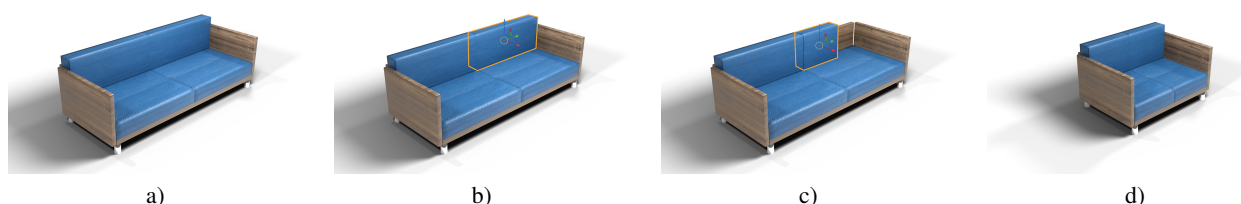
Figure 1: Pipeline of ADPM: The initial procedural model designed by a technical artist (a). The end user edits the model by shrinking the top right cushion (b-c). ADPM solves the inverse problem and propagates the modifications of the cushion back to the input parameters of the procedural model (d).
