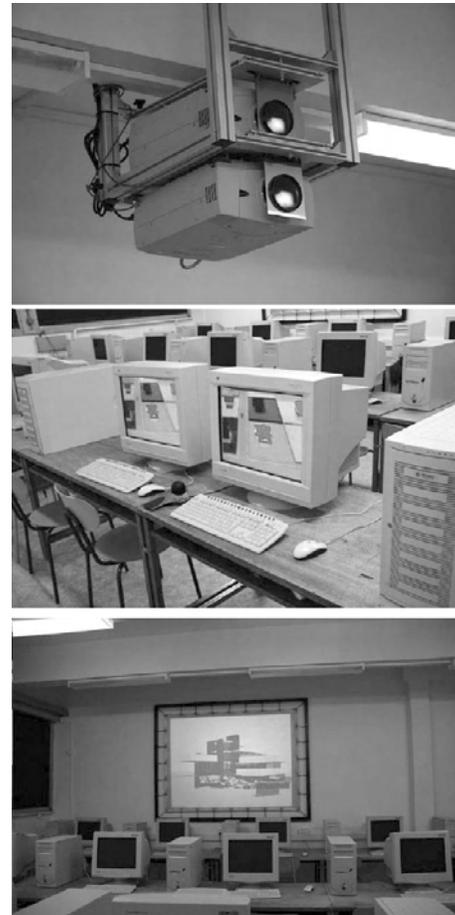
Figure 3: Hardware implementation. From top to down - projectors, dual PCs controlling the projection, projecting screen and the classroom
