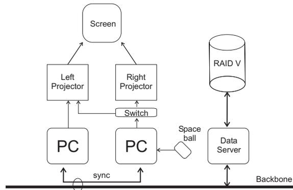
Figure 2: The Schema of the VR Center
