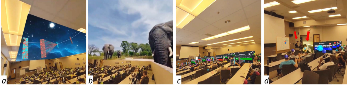
Figure 1: XRXL deployed in a large lecture with 82 students. The images are frames acquired with an XR headset from the back of the classroom, showing what the students see. The instructor has virtually retracted the ceiling to make room for a large-scale 3D visualization of a neural network (a). The instructor has turned the classroom into a 360° theater to take the class on an African safari (b). The instructor has partitioned the class into groups of four students, each with their own neural network 3D visualization and 2D panel for answering questions (c). The instructor pays a virtual visit to a group, without leaving the instructor's desk (d).
