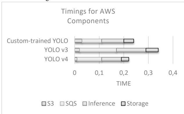
Figure 2. Time needed to process a video frame at each submodule of the framework (in seconds). S3, SQS, Inference and Storage represent what proportion of time a video frame spends at each step in the pipeline.
