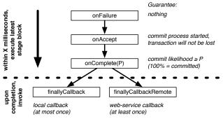
Figure 2: Client view of PLANET transactions
