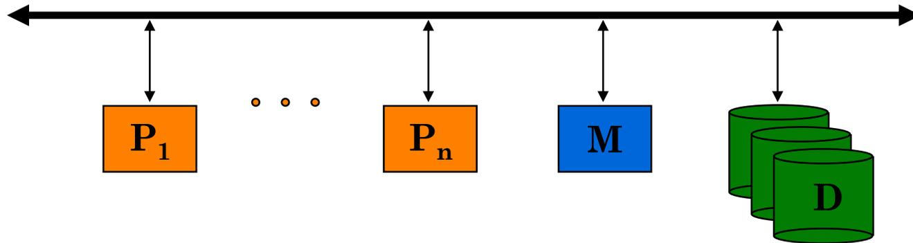
Examples : symmetric multiprocessors (Sequent, Encore) and some mainframes (IBM3090, Bull's DPS8)
