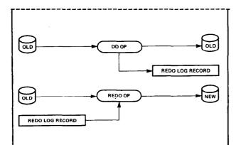
Figure 4. Real actions (ones that cannot be undone) must be deferred until commit. The logging approach to this is to apply the redo log of deferred operations as part of commit completion.
