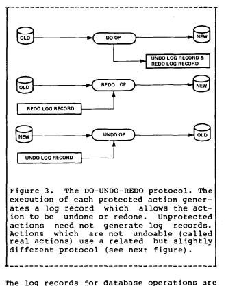
The fog fectors for database operations at very simple. They have the form: NAME OF TRANSACTION: PREVIOUS LOG RECORD OF THIS TRANSACTION: NEXT LOG RECORD OF THIS TRANSACTION: TIME: TYPE OF OPERATION: OBJECT OF OPERATION: OLD VALUE: NEW VALUE:
