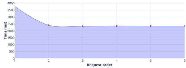
Figure 2: Parsing Module Azure Serverless Function Performance. The total time to execute the serverless function stabilizes after the second call.
