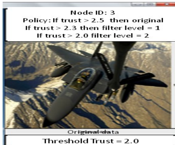
Fig.b. Policy of data sharing is at the top, original data in the middle and the virtual machine status at the bottom. Policy is based on the trust level of the AV: If above 2.5, original data is shared; if below 2.5 but above 2.3, minimal filtering is applied; if between 2.3 and 2.0 greater filtering is applied and if below the threshold of 2.0, no data is shared, in which case the active bundle destroys itself.
