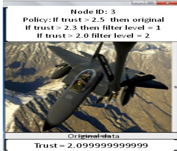
Fig.c. The trust level of the receiver AV is calculated as 2.09, which is higher than the threshold trust level, but not high enough to share the original data.
