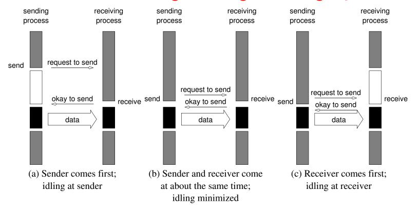
Handshake for a blocking non-buffered send/receive operation. It is easy to see that in cases where sender and receiver do not reach communication point at similar times, there can be considerable idling overheads.
