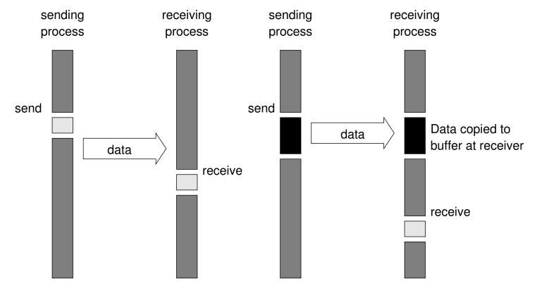
Blocking buffered transfer protocols: (a) in the presence of communication hardware with buffers at send and receive ends; and (b) in the absence of communication hardware, sender interrupts receiver and deposits data in buffer at receiver end.
