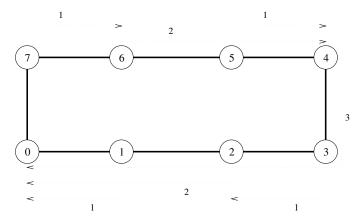
Reduction on an eight-node ring with node 0 as the destination of the reduction.
