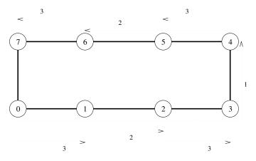
One-to-all broadcast on an eight-node ring. Node 0 is the source of the broadcast. Each message transfer step is shown by a numbered, dotted arrow from the source of the message to its destination. The number on an arrow indicates the time step during which the message is transferred.
