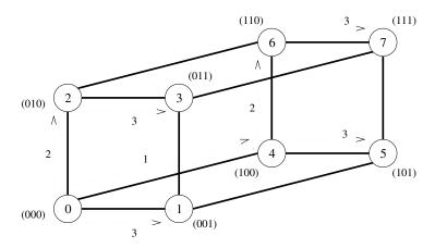
One-to-all broadcast on a three-dimensional hypercube. The binary representations of node labels are shown in parentheses.
