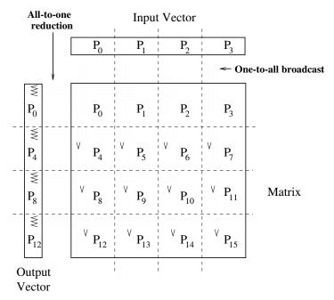
One-to-all broadcast and all-to-one reduction in the multiplication of a  $4 \times 4$  matrix with a  $4 \times 1$  vector.
