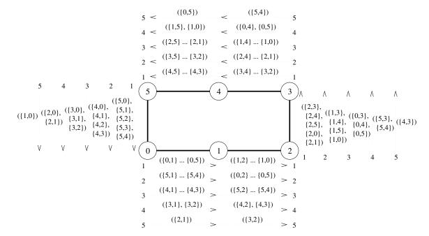
All-to-all personalized communication on a six-node ring. The label of each message is of the form  $\{x, y\}$ , where x is the label of the node that originally owned the message, and y is the label of the node that is the final destination of the message. The label ( $\{x_1, y_1\}, \{x_2, y_2\}, \ldots, \{x_n, y_n\}$ ) indicates a message that is formed by concatenating n individual messages.
