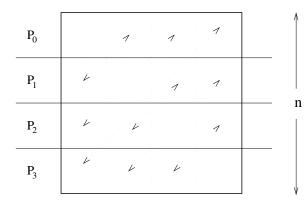
All-to-all personalized communication in transposing a  $4\times4$  matrix using four processes.
