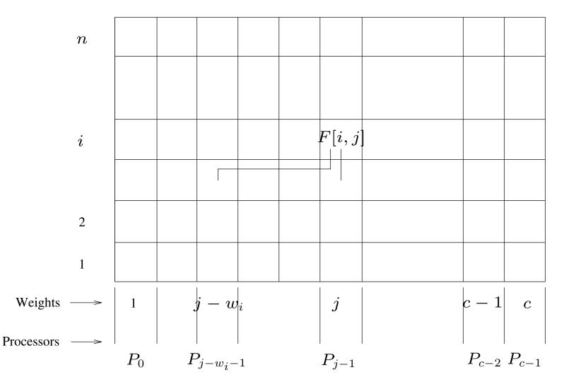
Computing entries of table F for the 0/1 knapsack problem. The computation of entry F[i, j] requires communication with processing elements containing entries F[i - 1, j] and  $F[i - 1, j - w_i]$ .
