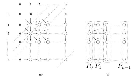
(a) Computing entries of table F for the longest-common-subsequence problem. Computation proceeds along the dotted diagonal lines. (b) Mapping elements of the table to processing elements.
