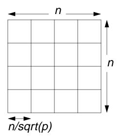
Each processor is assigned blocks of  $n/\sqrt{p} \ge n/\sqrt{p}$ . The algorithm proceeds in following steps:
