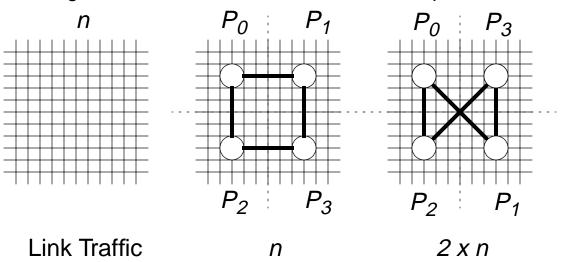
$\checkmark$  By making *n* large, the per-hop term can be masked, but in the second case, the bandwidth term is twice; in general it is *p*/2 times optimal. *It is all about bandwidth!!!*
