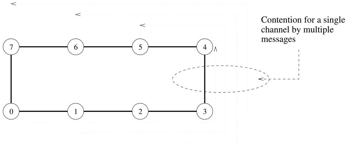
Contention for a channel when the hypercube is mapped onto a ring.
