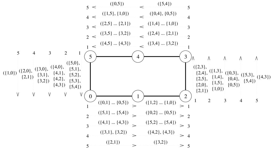
All-to-all personalized communication on a six-node ring. The label of each message is of the form  $\{x, y\}$ , where  $x$  is the label of the node that originally owned the message, and  $y$  is the label of the node that is the final destination of the message. The label  $(\{x_1, y_1\}, \{x_2, y_2\}, \dots, \{x_n, y_n\})$  indicates a message that is formed by concatenating  $n$  individual messages.
