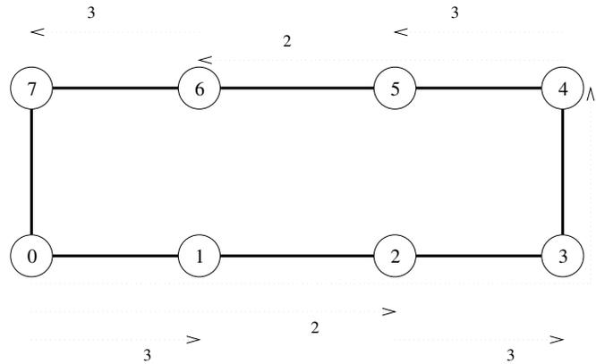
One-to-all broadcast on an eight-node ring. Node 0 is the source of the broadcast. Each message transfer step is shown by a numbered, dotted arrow from the source of the message to its destination. The number on an arrow indicates the time step during which the message is transferred.
