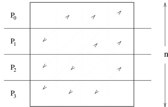
All-to-all personalized communication in transposing a  $4 \times 4$  matrix using four processes.
