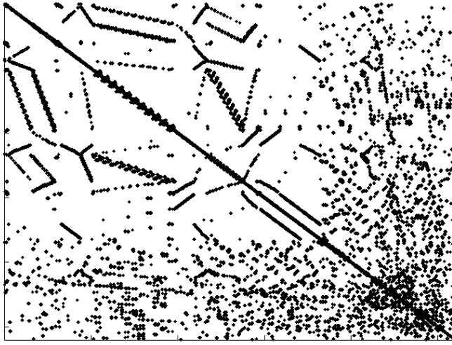
Fig. 9 Sparsity structure of the Hessian of the smallest mesh problem ( gear with n = 2,598 ).
