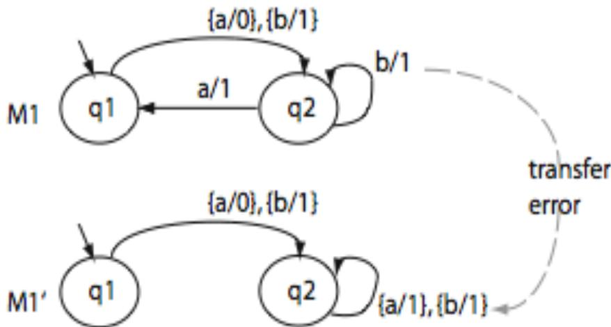
t=abba covers all states but does not reveal the error. Both machines generate the same output which is 0111.
