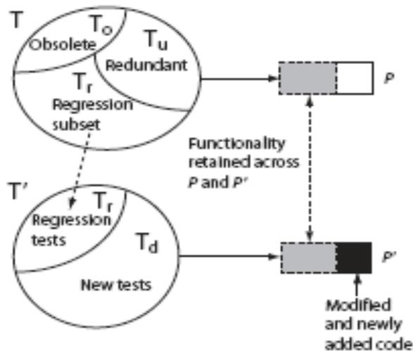
Note that some tests might become obsolete when  $P$  is modified to  $P'$ . Such tests are not included in the regression subset  $T_r$ . The task of identifying such obsolete tests is known as [test revalidation](#).
