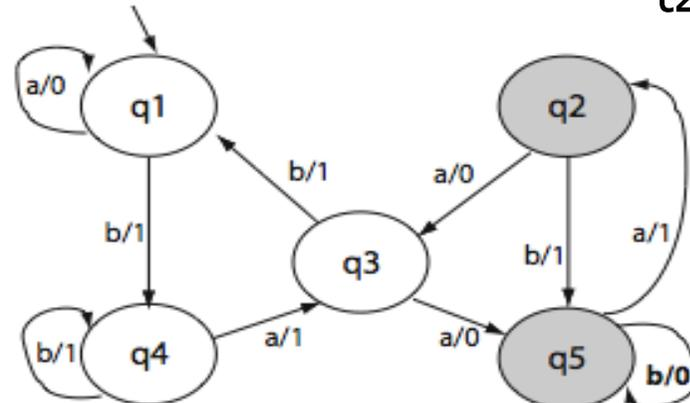
(c) Transfer error in state q2 and operation error in state q5.
