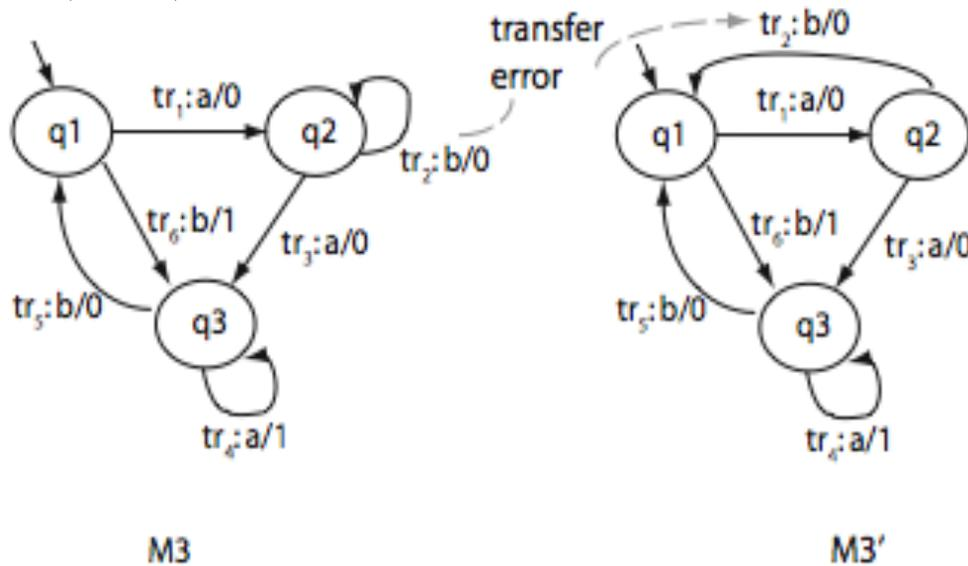
Consider  $T = \{t1: aab, t2: abaab\}$ . T1 causes each state to be entered but loop not traversed. T2 causes each loop to be traversed once.
