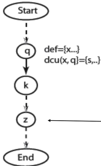
Path (Start, .. q, k, ..., z, .. End) covers the c-use at node z of x defined at node q given that (k ..., z) is def clear with respect to x
