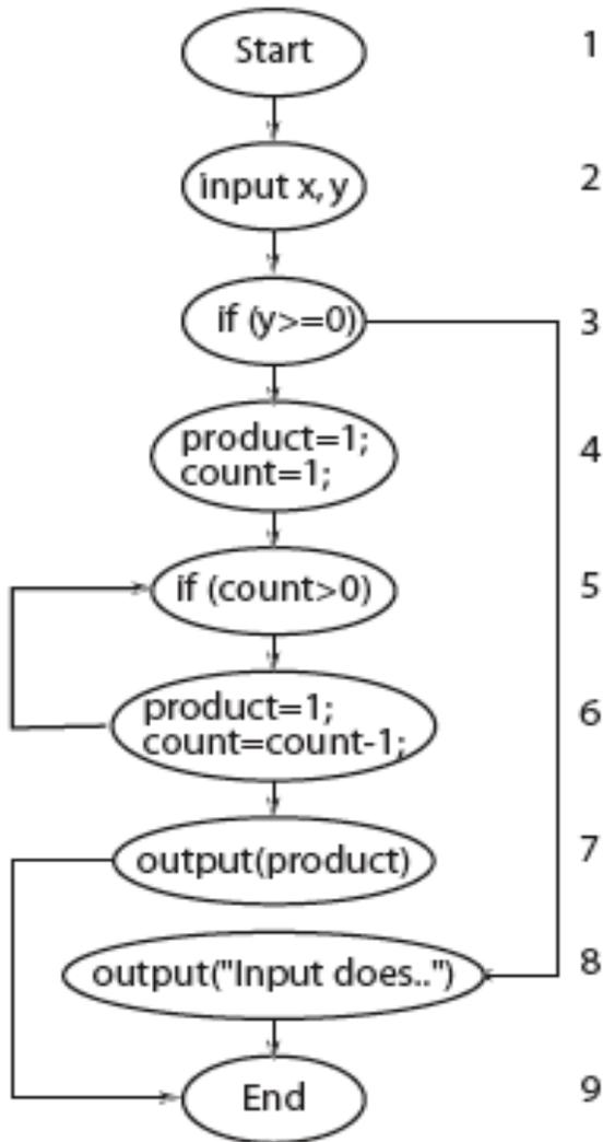
The modified path coverage criterion leads to  $C'_e = \{p_1, p_2, p_3\}$ . The elements of  $C'_e$  are enumerated below with respect to flow graph for the exponentiation program.
