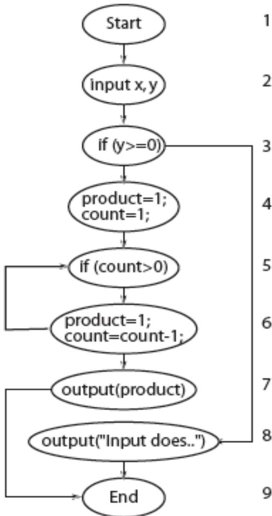
Any test case with  $y < 0$  will cause p3 to be traversed. Let us use  $t: \langle x=5, y=-1 \rangle$ . Test  $t$  covers path p3 and  $P$  behaves correctly. We add  $t$  to  $T$ . The loop in the enhancement terminates as we have covered all feasible elements of  $C_e$ '.
