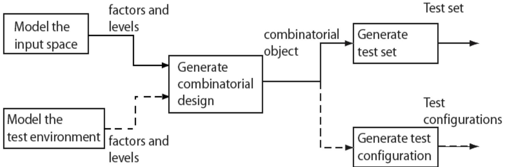
Modeling of input space or the environment is not **exclusive** and one might apply either one or both depending on the application under test.
