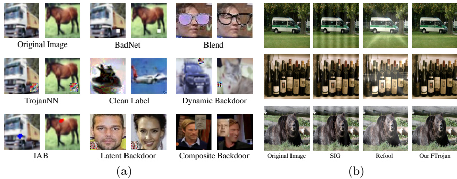
Fig. 1. The poisoning images of existing backdoor attacks. (a) Poisoning images from BADNET [20], Blend [11], TrojanNN [34], Clean Label [49], Dynamic Backdoor [41], IAB [37], Latent Backdoor [58], and Composite Backdoor [31]. (b) Poisoning images from SIG [7] and REFOOL [35].
