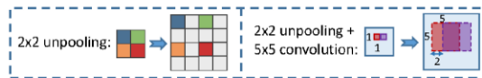
Figure 3. Illustration of unpooling (left) and unpooling+convolution (right) as used in the generative network.
