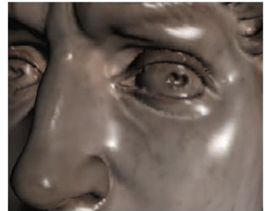
(c) Polygons – same number of vertices as (a) Twice the rendering time of (a)
