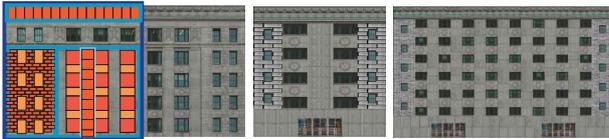
Figure 15. Left: The original facade picture partially overlaid with the grid structure, where blue frames and red grid cells are nested and random image layers, respectively. Middle and right: Two facades in that style at different sizes.
