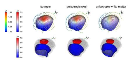
Fig. 9. Linearly interpolated EEG isopotential lines (in a blue–white–red scale) and MEG isofield lines (in a rainbow scale) (top row) and isopotential surfaces for  $-1 \,\mu$ V and  $7 \,\mu$ V (bottom row) for a mainly radially oriented source in somatosensory cortex: isotropic model (Left), 1:10 anisotropic skull using the volume constraint (middle) and 1:10 anisotropic white matter using the volume constraint (right).
