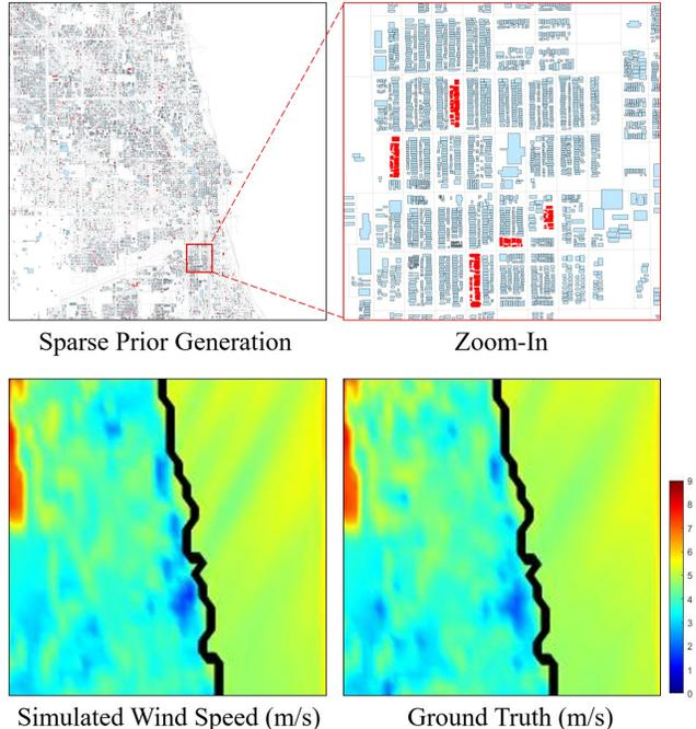
Figure 5: **Sparse Prior Generation.** Top: we show a generated Chicago from only 5% prior data (shown in red), and a Zoom-In. Blank areas indicate non-building structures (e.g., parks, rivers, roads). Bottom: generated layout used by a local weather forecasting model [9] yields almost identical wind speed simulation compared to the ground truth.
