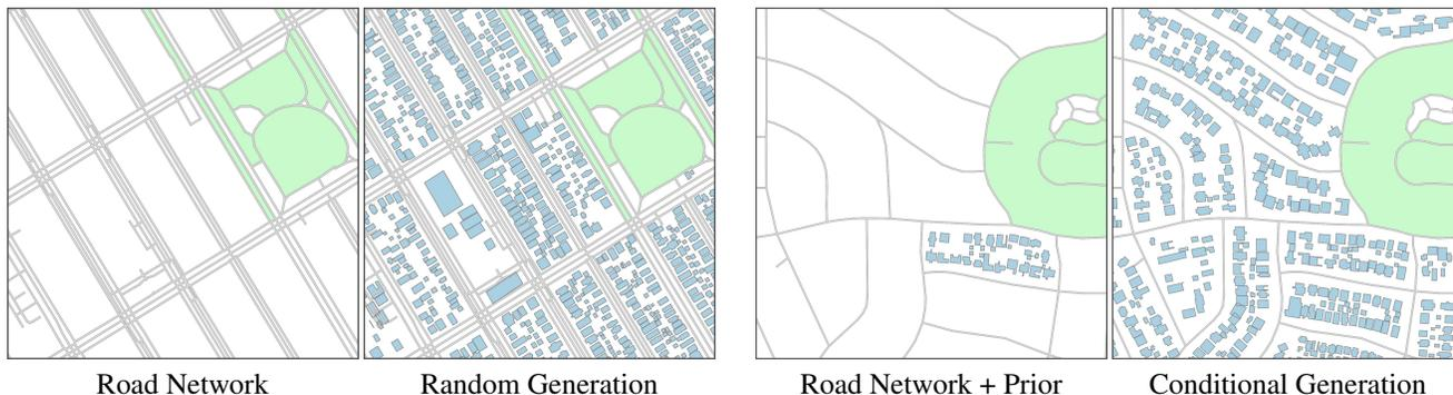
Figure 1: **Arbitrary Urban Layout Generation.** Our method generates realistic urban layouts given an arbitrary road network (Left Pair). Moreover, given learned prior from a building layout, our method conditionally generates similar urban layouts for the given arbitrary road network (Right Pair).
