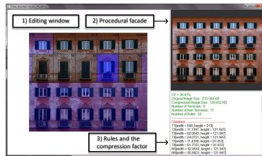
Fig. 2. The user represents the original facade (1) as a procedural representation. The application shows the result in the second window, while the third window (3) shows the procedural rules and the compression factor.
