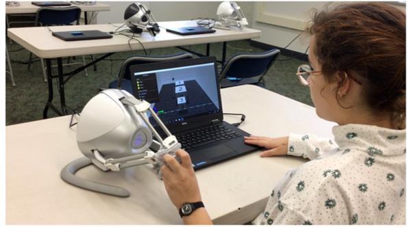
Figure III.2 User manipulates with the haptic device and the system provides visual and tactile feedback.
