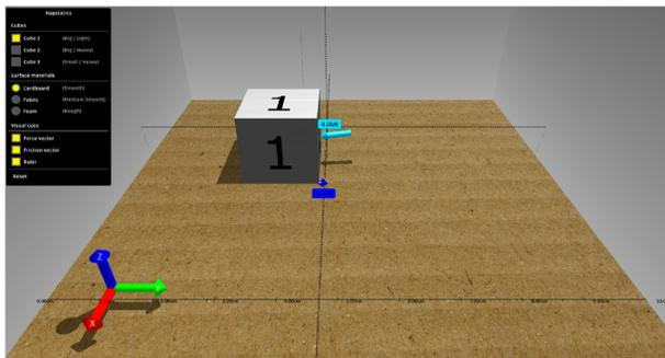
Figure III. 1: Visuo-haptic simulation shows the coordinate system, the 3D cross-hair cursor, and the applied force
