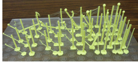
Figure 5: An example of the printed test setup used to find the value of \alpha_c and the optimal length of supporting strut.
