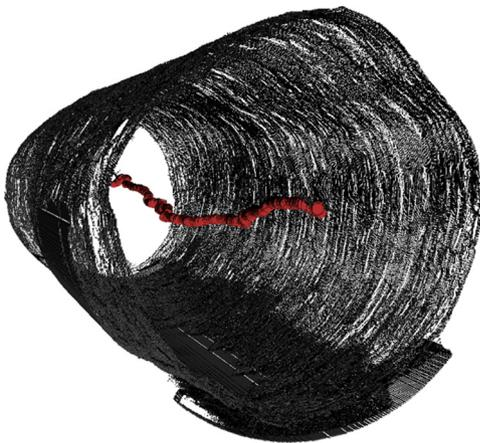
Fig. 3. Visualization of pith in 3D showing its location along entire log.
