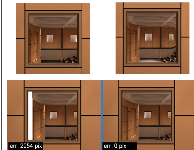
Figure 21 Auditorium seen through a square portal (window). ( Top ) Depth image ( left ) and OCRI ( right ). The OCRI essentially enlarges the portal and captures more samples inside the auditorium, which are then used to prevent disocclusion errors. ( Bottom ) Frames rendered from DI ( left ) and OCRI ( right ).
