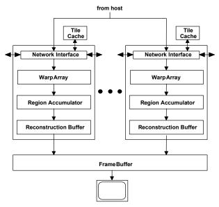
Figure 3. Block diagram of the *WarpEngine*
