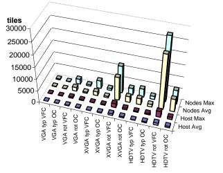
The host bandwidth required can be supplied by the AGP interface, as all maximum host-to-*WarpEngine* communication volumes are below 4 Ktiles. The Network Interface that interconnects the nodes is not fully designed yet; from experience we are confident that ring bandwidths of 8 to 64 Gb/s are attainable. At 60Hz this translates into 8 to 64 Ktiles / frame which from the above graph appears to be sufficient for the highest node-to-node traffic.
