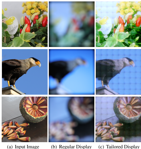
Figure 12: Input images (a) and how they are perceived on a tailored display by a farsighted subject (c). The HMD prototype was placed t = 20cm from the eye (camera). The camera simulated a subject whose closest focal point is j = 50cm (subject using +3D lenses). Picture (b) shows how the subject sees the respective image on (a), with same size, at the same distance in a standard monitor. Since our setups have small spatial resolution, we mimicked an array of LCDs by changing the image being displayed to cover a bigger "retinal" area. (b) is a collage (sum) of 64 square patches which create a 3.4 arc-minute image on the retina (each path = 0.425 arc minutes). The blue channel of (c) was adjusted to 75\% of its captured intensity to remove prototype light leaking.
