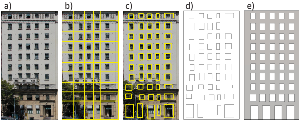
Figure 4: Façade Generation. a) Given the façade image, b) our approach uses a CNN to find the initial estimate of floor and column boundaries which are refined by the image-based approach. c) Then, for each tile image, window recognition CNN and window parameter estimation CNN are used to detect windows, and d) a simplified façade image is generated. For the façade region excluding the window region, a dominant color is calculated as a façade color. e) Finally, the façade recognition CNN and façade parameter estimation CNN are used to recognize the façade style and estimate parameter values for the selected façade grammar.
