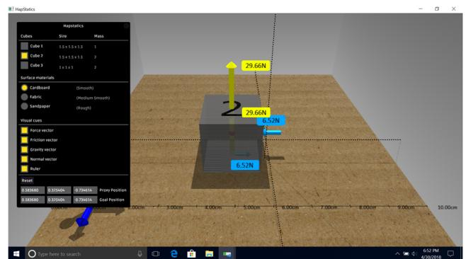
Fig 5 Free body diagrams and the visuo-haptic simulation
