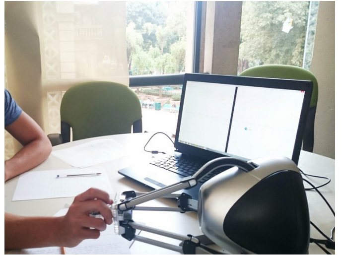
Fig. 4. A student interacting with the Plane Charge simulator. Students can freely explore the virtual scenario by using a haptic device. Depending on the position of the haptic interaction point, students can feel the interaction force in that position.
