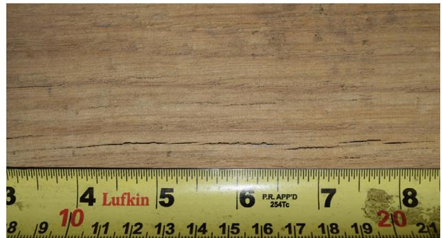
Fig. 6. Surface checks in white oak board.
