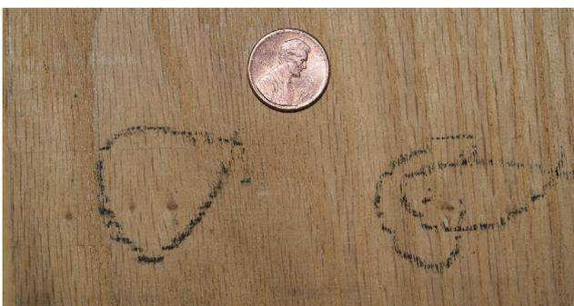
Fig. 3. Pin knots in red oak board.
