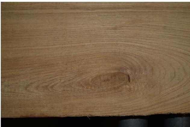
Fig. 2. Large pale knot in ash board.
