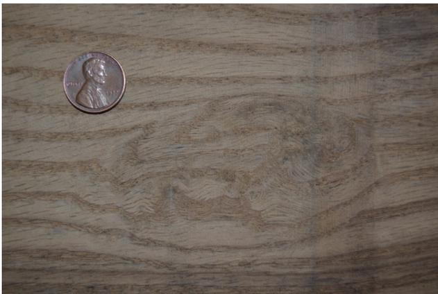
Fig. 5. Burl detected as a knot in red oak board.
