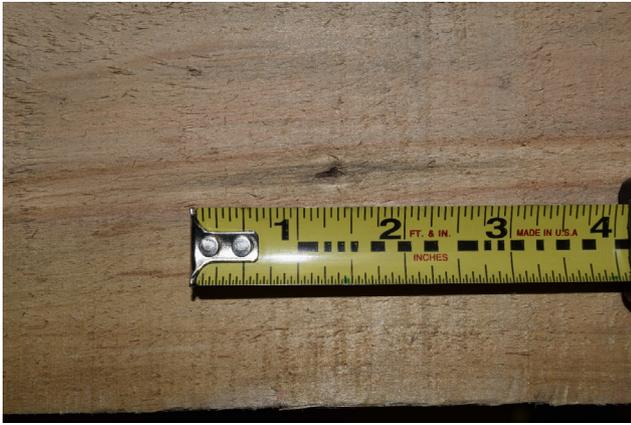
Fig. 11. Worm hole in soft maple board.
