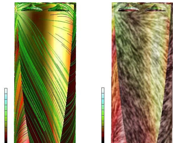
Fig. 1 The visualization of swirl motion at the inner boundary surface of a combustion chamber from an automotive engine cylinder: (left) geometric flow visualization using streamlines, and (right) texture-based flow visualization, both being used in combination with velocity magnitude color-map.
