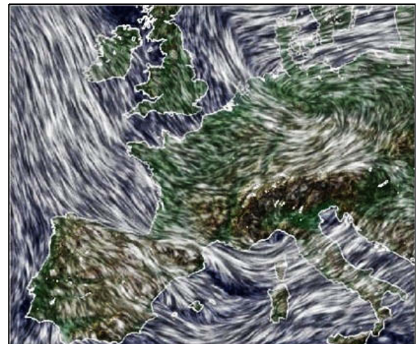
Fig. 2 The time-dependent weather patterns over Europe. This visualization is the result of the Lagrangian-Eulerian Advection (LEA) algorithm (Jobard, Erlebacher and Hussaini, 2002). Data courtesy of the Swiss Center for Scientific Computing ( http://www.cscs.ch/index.php?option=com_content&task=view&id=99&Itemid=133 ).
