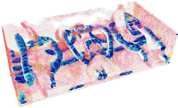
Fig. 8 3D visualization of Benard convection. Benard convection leads to an exchange of heat between a hot bottom surface and a colder top surface.
