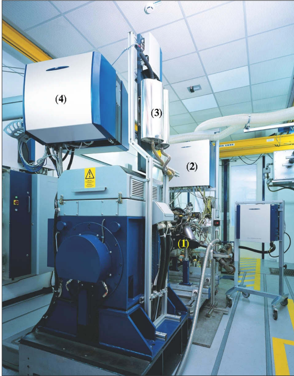
Fig. 4 Monitoring equipment is hooked up to a running engine and catalytic converters: (1) the running engine, (2) connected measurement equipment, (3) the exhaust system, and (4) equipment measuring and monitoring the exhaust system. This measured data is compared to CFD simulation data. Photo courtesy of AVL.
