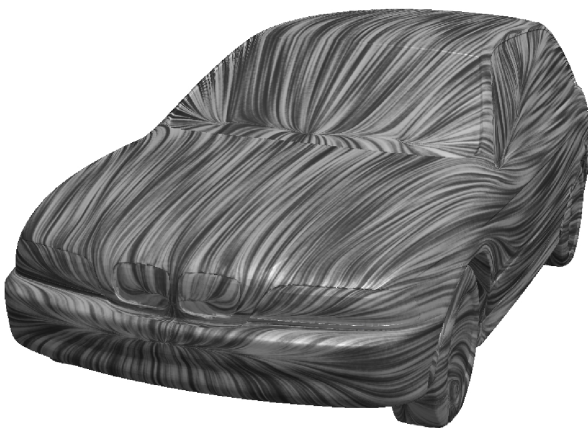
Fig. 7 Texture-based flow visualization on a curved surface for an automotive CFD simulation.
