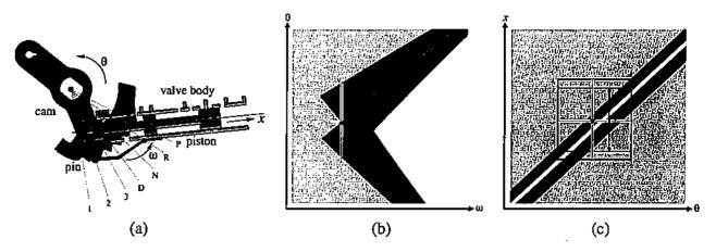
Figure 10: (a) Gear selector; (b) pin/cam contact zone; (c) cam/piston contact zone.
