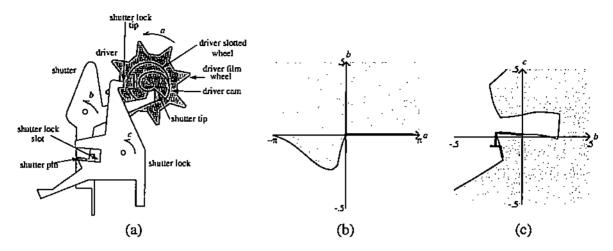
Figure 14: (a) Camera shutter mechanism; (b) driver/shutter configuration space; and (c) shutter/lock configuration space with motion path.
