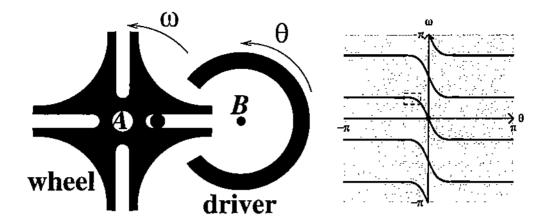
Figure 1: Geneva pair and its configuration space.
