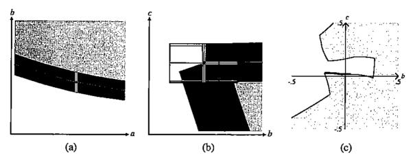
Figure 15: (a) driver/shutter contact zone detail; (b) shutter/lock contact zone detail; (c) failure in shutter/lock configuration space.
