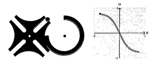
Figure 6: Jamming Geneva pair and its configuration space.
