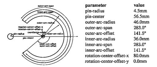
Figure 3: Parametric model of Geneva driver.
