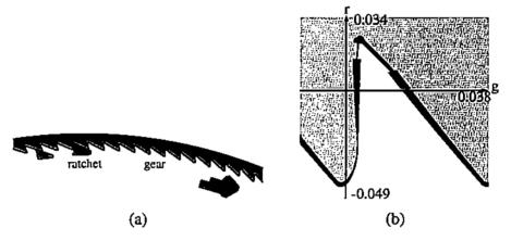
Figure 13: (a) Gear/ratchet pair; (b) contact zone.
