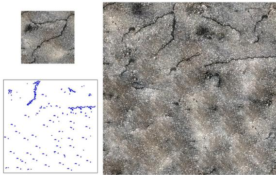
**Fig. 8** An automatic synthesis using a simple procedural model. From the input (top left), extracted edge groups are automatically distributed (bottom left) based on the procedural representation. The bottom one-third of the output (right) does not have the crack patterns, whereas the rest shows mixed structures
