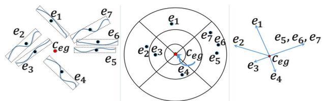
**Fig. 5** Edge group representation. Each edge group has its center  $c_{eg}$  and a set of edges ( $e_1, e_2, \dots, e_7$ ) (left). The edge centers are discretized into a grid in polar coordinates centered around  $c_{eg}$  (middle). The edge group is represented by the non-empty cells (right), and each cell stores its distance from  $c_{eg}$ , the angle, and the list of corresponding edges
