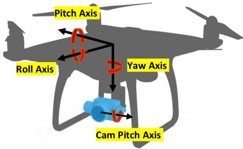
Fig. 5. Drone coordinate system.
