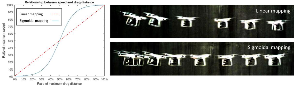
Fig. 6. Linear mapping of the velocity and the drag distance cause the drone to move abruptly and sway at the beginning and at the end of each gesture (top right trajectory). We compensate for this behavior by using a sigmoidal function, and the corresponding trajectory is shown on the bottom right.
