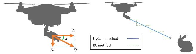
Fig. 7. Our unified control of the drone motion and camera motion allows for a smooth transition between the motion and camera aiming.
