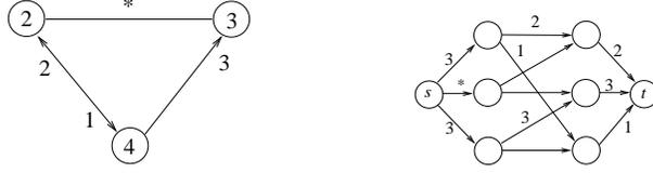
Figure 4: Current graph  $G'$  and corresponding network  $G^*$ , the edge marked by asterisk is currently being distributed
