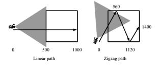
Figure 2: Camera paths through the scene. The square represents the scene dimensions, gray area represents the viewing frustum and frame number has been written at key positions.
