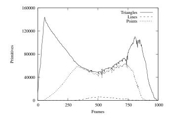
Figure 6: Rendered primitives during the linear camera path using TCLOD implementation with a target time  $t_f = 0.04sec$ .
