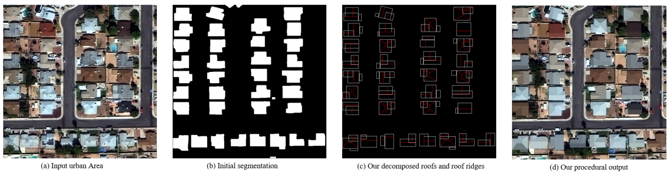
Figure 1: Our method automatically generates procedural roofs for an input urban area. (a) An input urban area from SpaceNet dataset [VLB18]. (b) The initial segmentation (Mask R-CNN [HGDG17]) of (a). (c) Our decomposed roof parts and predicted ridges. (d) Our generated procedural roofs rendered on top of real image (a).
