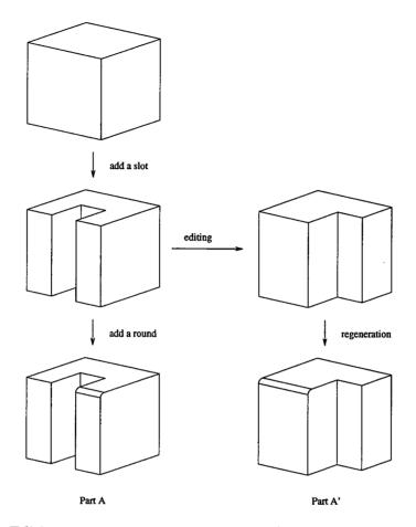
Figure 2: Editing example 1: When the slot (second feature of Part A) is moved to the right and becomes a step, rounding the edge in Part A' should be considered an error.
