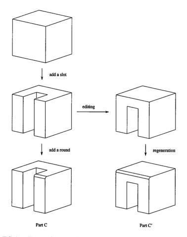
Figure 4: Editing Example 3: When the through slot (second feature of Part C) is changed to a blind slot, the entire edge of Part C' should be rounded. For subsequent editing Parts B and C' should be equivalent.
