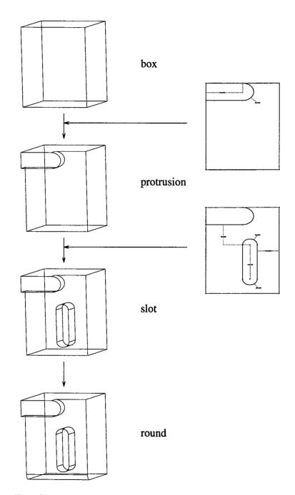
Figure 5: Erep feature construction: A part is created with a block, a protrusion, a slot and a round. The features were added sequentially. Cross sections are shown to the right.
