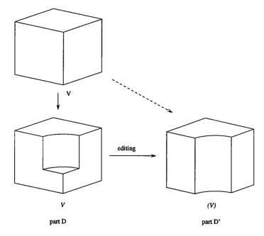
Figure 8: The vertex V of part D is not found in part D'. As a proto feature vertex, it can be reconstructed from the first feature of part D'.
