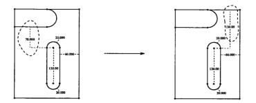
Figure 6: The slot dimensioning schema is edited. The new schema shown to the right no longer references the protrusion, so the slot position is now independent of the protrusion feature and its variations.
