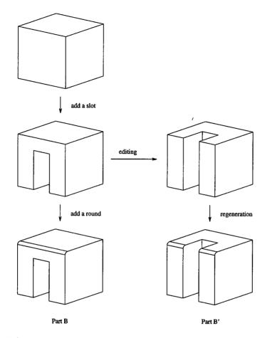
Figure 3: Editing example 2: When the slot (second feature of Part B) is moved to the right and becomes a step, rounding the edge in Part B' should be considered an error.
