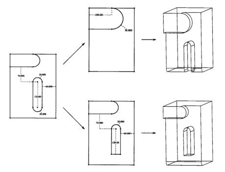
Figure 7: Top: Using the dimensioning schema left, editing the protrusion radius will affect the position of the slot feature.
