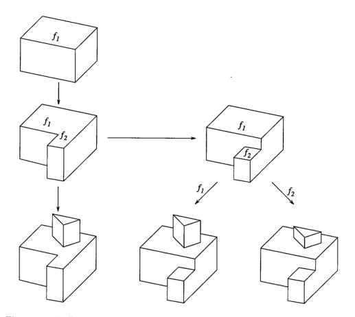
Figure 11: Different representatives of a merged face produce different results after feature editing.
