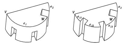
Figure 10: Left: Edge  $e_1$  is named in the design. After editing, the edge is subdivided by colliding features. Segments  $e_{11}$ ,  $e_{12}$ , and  $e_{13}$  match.
