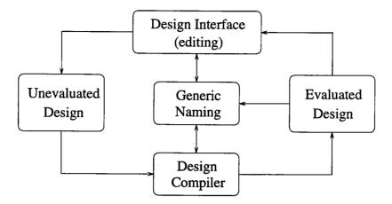
Figure 1: A design model is layered into an unevaluated representation and an evaluated representation.
