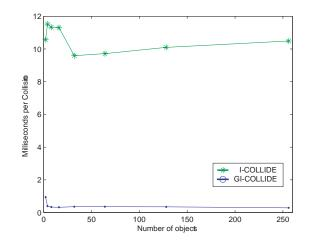
Figure 9: Average time needed to detect a collision for I-COLLIDE and GI-COLLIDE
