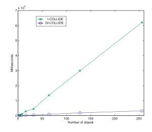
Figure 8: Time spent for collision detection with I-COLLIDE and GI-COLLIDE
