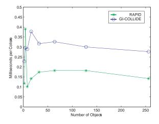
Figure 11: Average time needed for collision detection by RAPID and GI-COLLIDE
