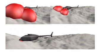
Figure 2: Sphere hierarchy refinement during the collision detection
