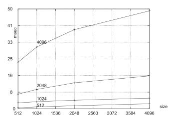
Figure 12: Number of collision tests as the function of object resolution. Two equal objects in varying resolution are colliding and the collision detection times are reported. The lines show the tests performed with geometry images in resolution  $513^2$ ,  $1025^2$ ,  $2049^2$ , and  $4097^2$
