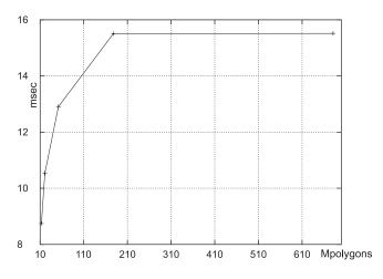
Figure 13: Time required for the collision test as the function of object resolution in the case of time critical collision detection. Object in resolution  $2049^2$  was tested against objects in resolution  $513^2$ , ...,  $8193^2$ . The framerate was kept on 60 fps. The *x*-axis shows the number of millions of polygons tested, the *y*-axis the time in milliseconds required to find the first collision
