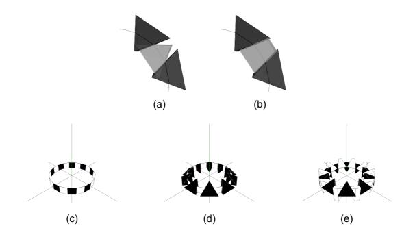
Figure 1: TIC generation on a cylinder: (a) Generated pieces using the original method, (b) Quasi tetrahedron between two regular tetrahedra, (c) Ring of squares following the polygonal approximation of the cylinder, (d) Regular tetrahedra generated from black squares, (e) Quasi tetrahedra pieces generated from white squares. A single ring is shown for visualization purposes.
