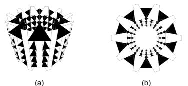
Figure 2: TIC based on a cylinder with radius 10, 20 pieces per ring and 5 rings: (a) Perspective view, (b) Top view.
